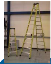
Photo 1: This experiment used 6-ft and 12-ft Type 1A fiberglass ladders.
