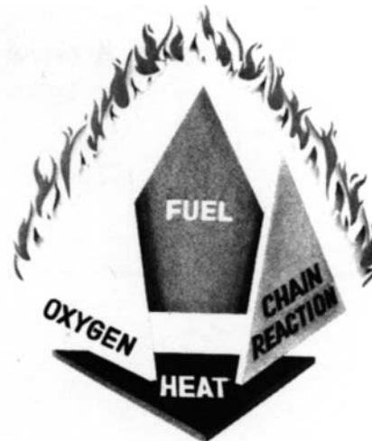
Figure 9. The fire pyramid, which illustrates the four factors necessary for a fire to exist. Remove any one of the four and the fire is extinguished.
