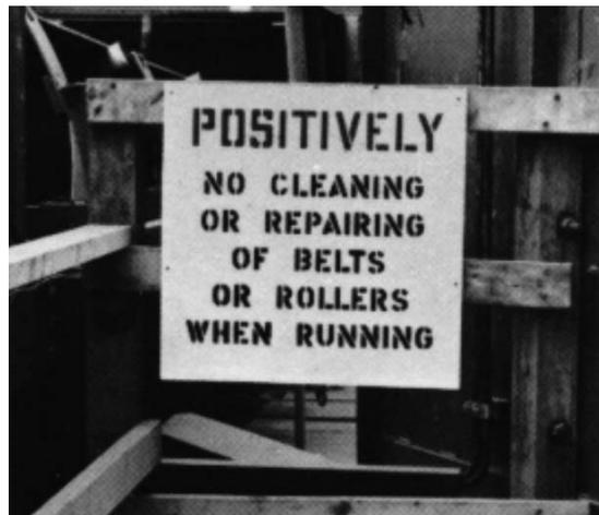
**Figure 4.** Signs, such as the one shown, should caution workers against unsafe practices around belt conveyors.
