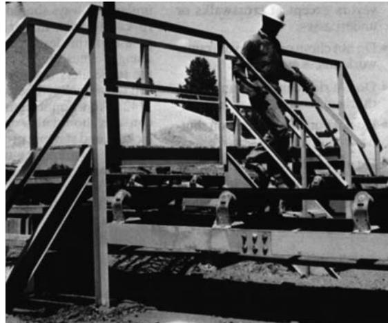
**Figure 3.** Workers must cross conveyors only at crossovers or underpasses and should be prevented from crossing elsewhere.
