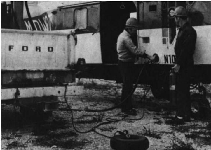
**Figure 7** shows a typical helicopter refueling takes two workers, one to handle the refueling and one to stand by in case of fire. Note the bonding between the truck, from which the fuel is pumped, and the helicopter. The helicopter is grounded with a metal stake driven into the earth.
