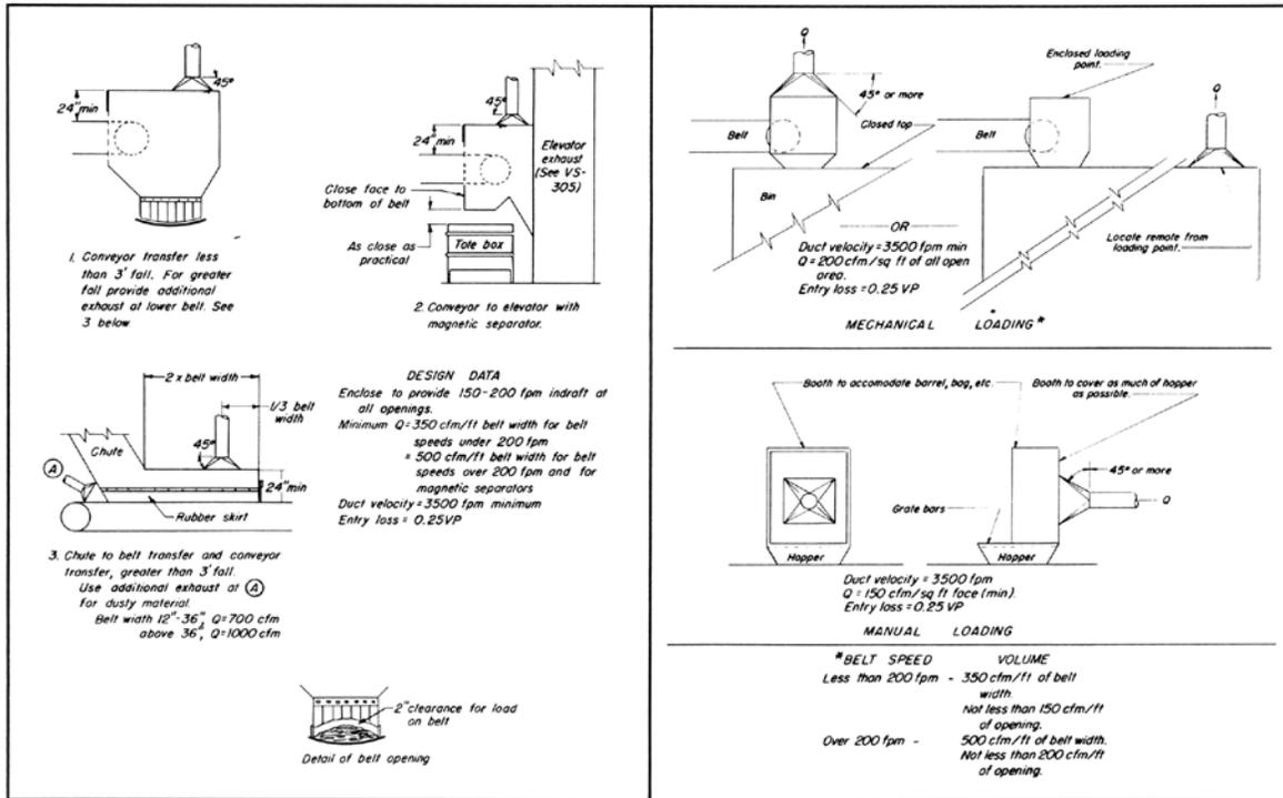
**Figure 2.** Left: Suction hoods at belt loading and discharge points control nuisance dust. Right: Bin and hopper ventilation will stop dust problems. Note: Air velocities indicated are minimum standards. (Drawings courtesy Industrial Ventilation, published by ACGIH).
