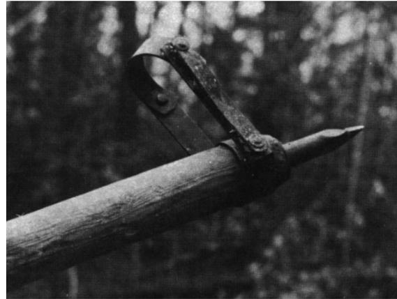
**Figure 3.** This specially designed tree hook is used to control a tree being cut. The spear end is plunged into the tree trunk, and the other end is held on the ground. As the tree is cut, the trunk is guided away from the chainsaw operator.
