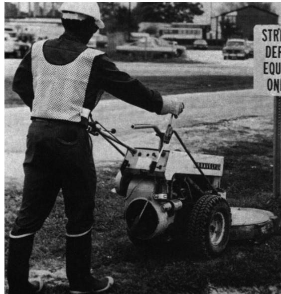
**Figure 2.** This properly dressed hand-mower operator wears boots, gloves, safety glasses and a helmet. The addition of a brightly colored vest makes him highly visible to motorists.
