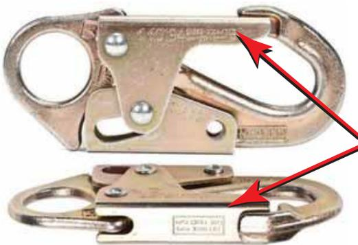
All acceptable snap hooks or carabiners have a kilo-Newton (kN) rating engraved into the spine. Since 2007, the newest ANSI standard requires all fall protection hardware to have a minimum 16 kN (3,600 pounds) rating for the gate and 22.5 kN, (5,000 pounds) tensile load (ANSI Z359.1-2007, Section 3.2.1.4.). (A kilo-Newton equals about 225 pounds, which is a force of gravity and not static weight or mass. Force = mass times acceleration.)
