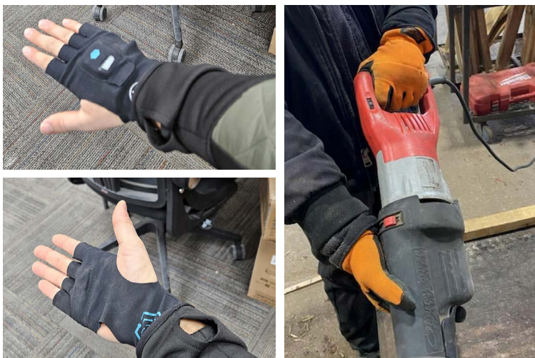
Figure 6. Image depicts an individual wearing the HAV-Sentry glove and completing a task
